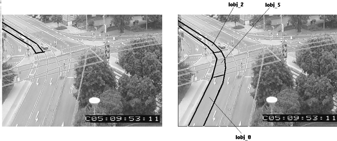
Figure 2. The left panel shows an image frame from the sequence illustrated in Figure 1, overlaid by the lane model for this intersection. One lane segment of the ‘incoming’ lane entering the field of view from the top left corner is marked by heavy boundary lines. The right panel exhibits the same image, but this time the ‘intersection crossing’ segment and the ‘outgoing’ segment of this same lane are marked by heavy boundary lines, too. In addition, the lane identifiers for the three segments of this lane are given.
